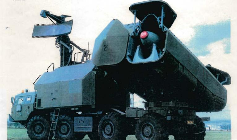
This picture shows the launcher automatically being trained round to the firing bearing. The PLANKSHAVE is in sector scan and the target is being tracked in auto.
