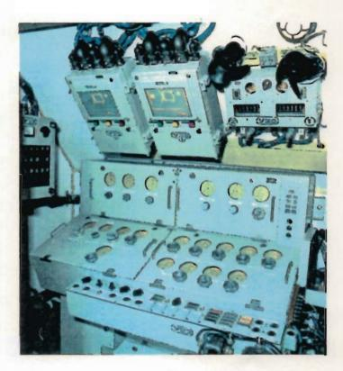
The launch console operator controls the information fed to the missiles through the analogue launch computer. Target information is normally provided by a third party using secure voice – this is manually put into the launch computer or automatically entered if the information is from PLANKSHAVE. The operator then selects the missile flight profile, chooses the missile to be fired, puts the launcher to cuto and fires the missile in sequence with the other TELARS.
